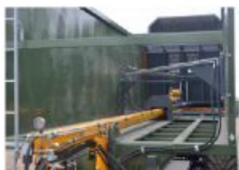
Hydraulic system of sliding wall
